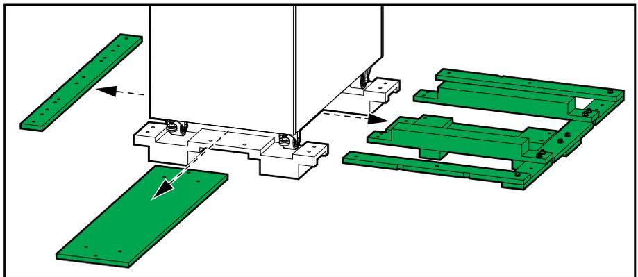
5. Use a forklift to lift the UPS and remove the remaining pallet parts.
