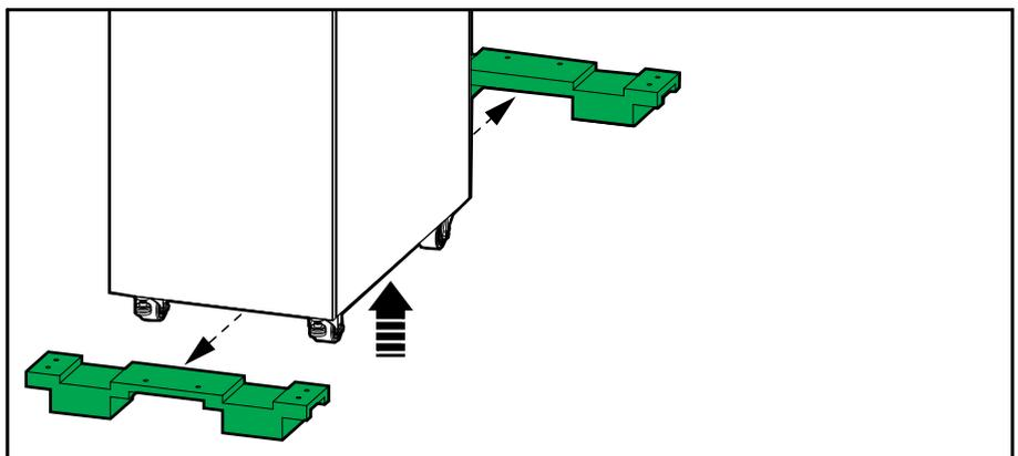
6. Move the UPS to its final location and use a wrench to lower the levelling feet. Ensure that the cabinet is level.
