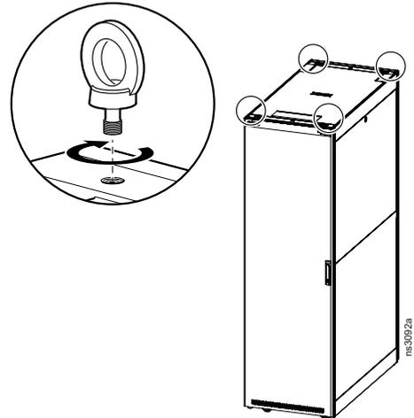
Assure a straight-line pull on the lifting eye bolts when lifting the Easy Rack.
