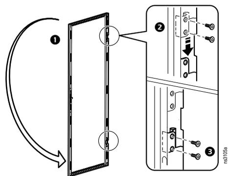
Install the door to the hinges now on the reverse side of the rack. Connect the ground wire and any other wire connections previously disconnected.
