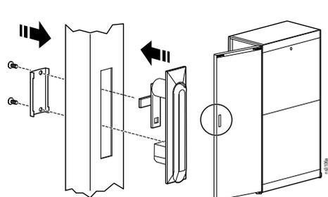
Rotate the cam washer 90 degrees, and the latch 180 degrees. Install the handle on the door.
