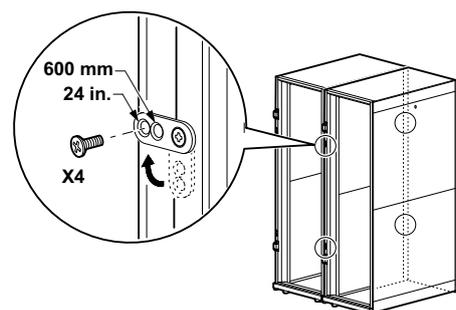
Install the doors. See the “Door Installation” section for instructions.
