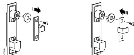
Locate the lock handle. Remove the cam screw, cam washer, and cam.
