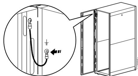
Locate the upper hinge on the rack frame. Remove the two screws holding the hinge in place. Install the hinge onto the other side of the rack frame. Repeat this step for the lower hinge.
