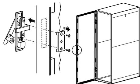
Disconnect the ground wire, and any other connections. Remove the door from the frame.
