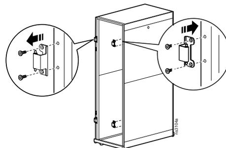
Rotate the door. Remove the hinges from the door, and install them to the alternate hole location. The hinges on the door should now align with the hinges on the rack.
