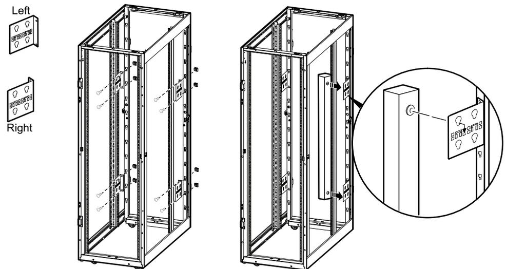
The Easy Rack is shown with doors and side panels removed for clarity.
